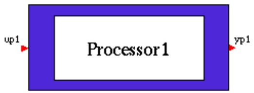
The Processor Block represents the final target in which your software will be installed. It collects one or more schedulable control functions running on a single processor (mono or multicore).
