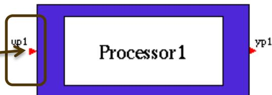
By inserting a Processor Input Block you introduce a new input in the Processor Block.
