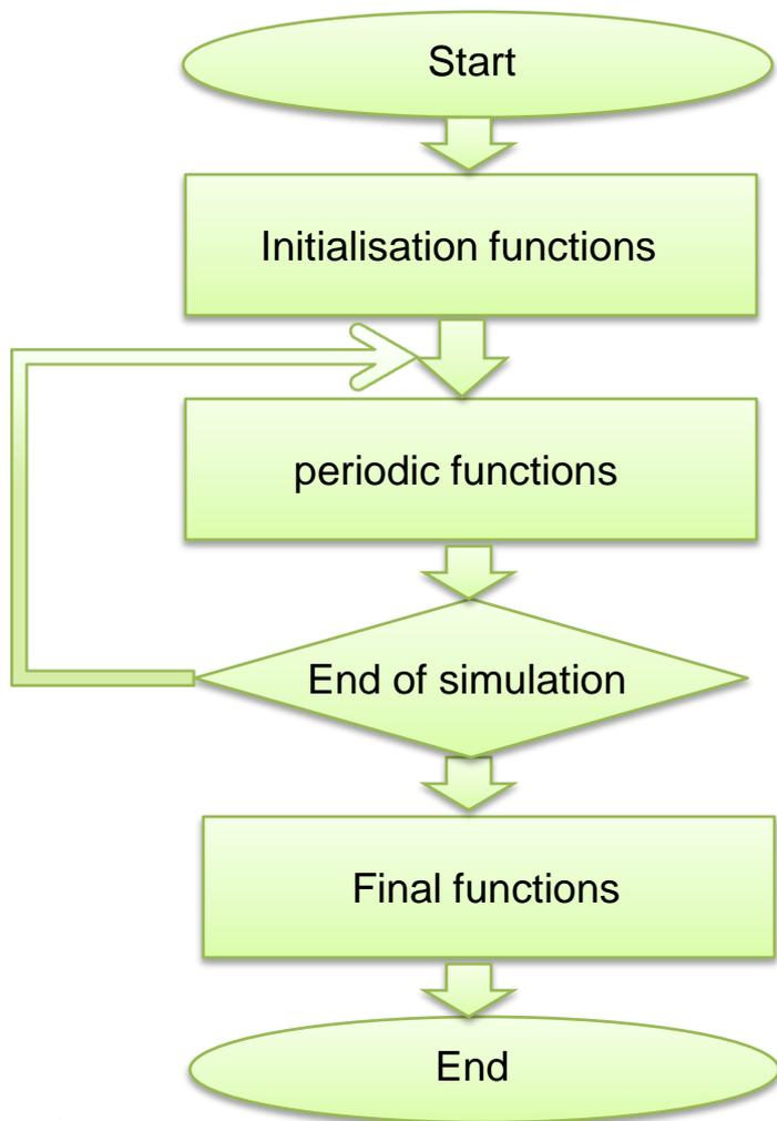
The EICASLAB scheduler performs a simulation with period equal to the simulation step.
