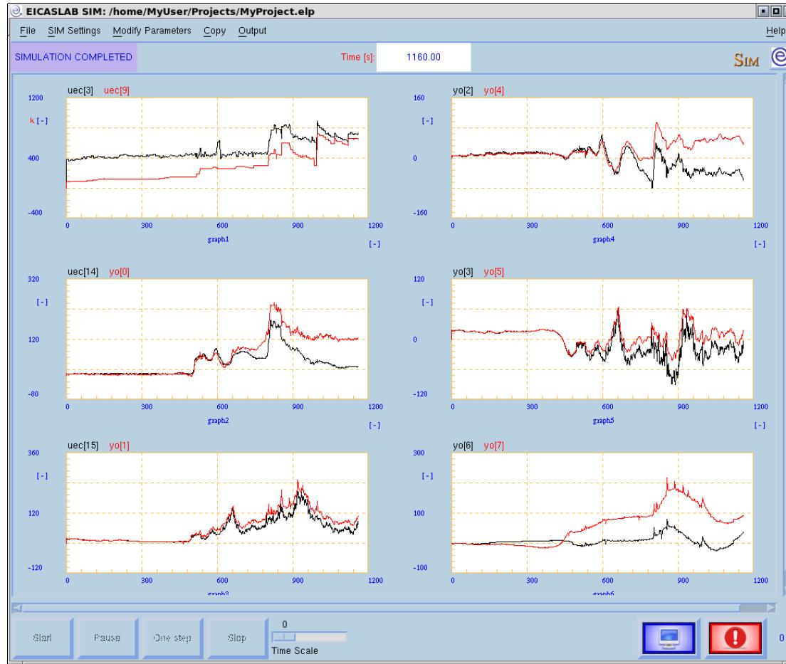
In the first step, a preliminary simulation - called **initial Base Trial** - is performed starting from the initial parameter values provided by the user and a preliminary evaluation of the *cost function* is made.
