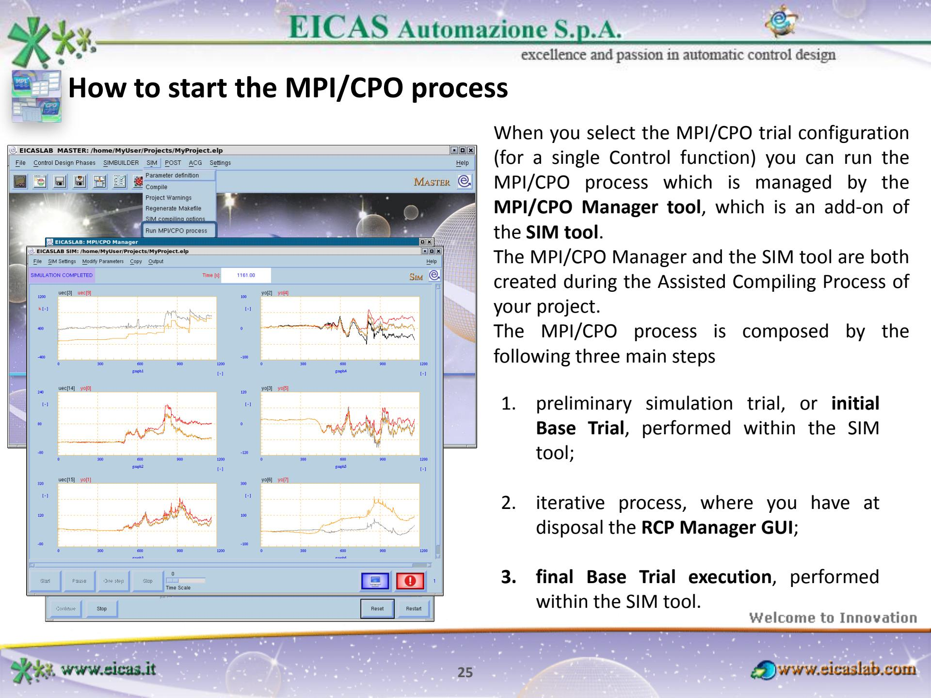
When you select the MPI/CPO trial configuration (for a single Control function) you can run the MPI/CPO process which is managed by the **MPI/CPO Manager tool**, which is an add-on of the **SIM tool**.
