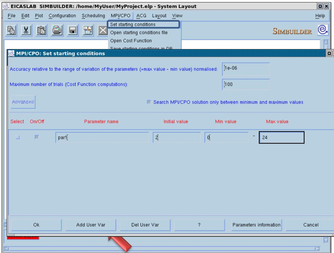
You can select the parameters to be identified/optimised through the “*Set Starting conditions*” window, clicking on the “*Add User Var*” button.
