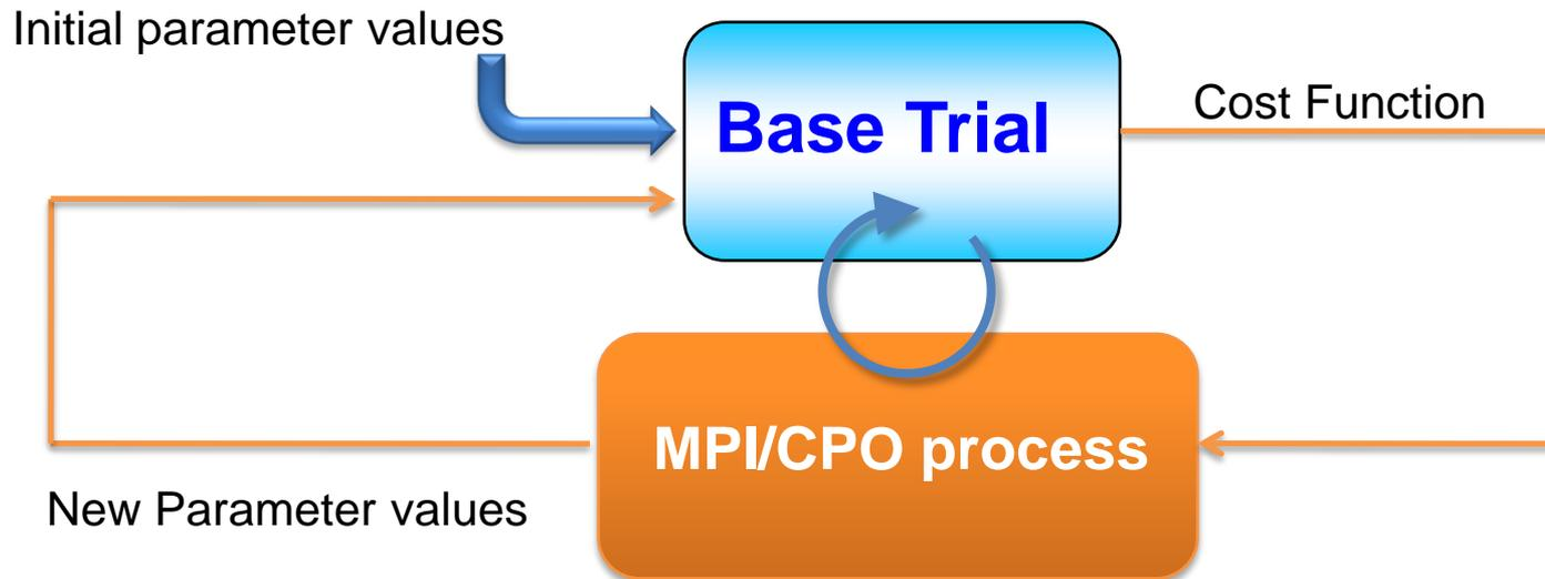
1. During the initial Base Trial a preliminary simulation is performed starting from the initial parameter values provided by the user and a preliminary evaluation of the *cost function* is made.
