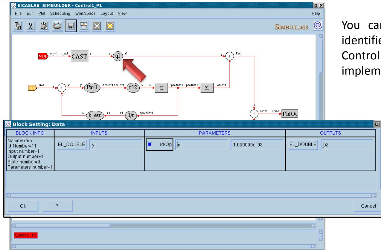
You can select the parameters to be identified/optimised directly in the Control Graphical Layout where you have implemented your control algorithm.
