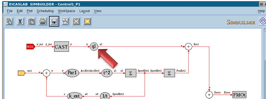
You can select the parameters to be identified/optimised directly in the Control Graphical Layout where you have implemented your control algorithm.
