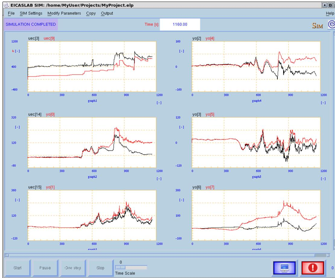
In the first step, a preliminary simulation - called **initial Base Trial** - is performed starting from the initial parameter values provided by the user and a preliminary evaluation of the *cost function* is made.
