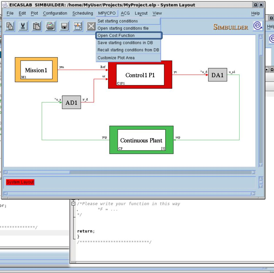
When you select the MPI/CPO for a Graphical Control, a special block, named “*FltDt*”, is automatically inserted in the Control Graphical Layout.
