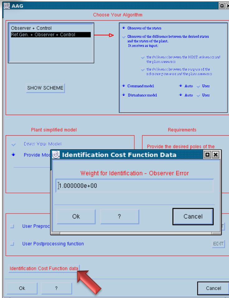
For the AAG Controls EICASLAB manages automatically the *cost function* used in the MPI process.
