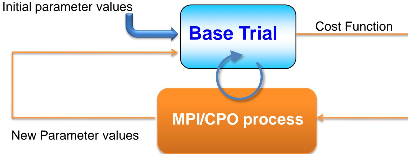
1. During the initial Base Trial a preliminary simulation is performed starting from the initial parameter values provided by the user and a preliminary evaluation of the *cost function* is made.
