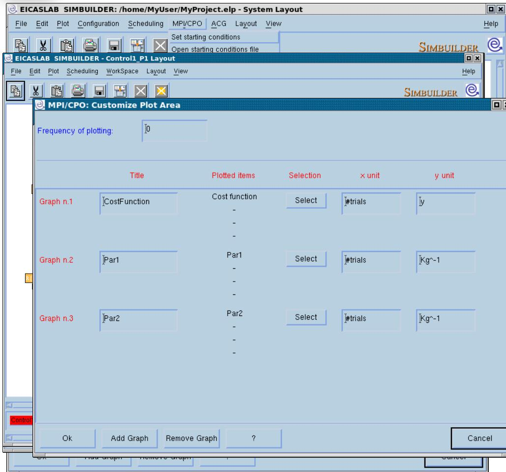
Before running the MPI/CPO process, you can customise the related plotting windows by means of the “Customise Plot Area” menu which allows you to quickly select which parameters to display during the MPI/CPO process (you can also display the cost function) .
