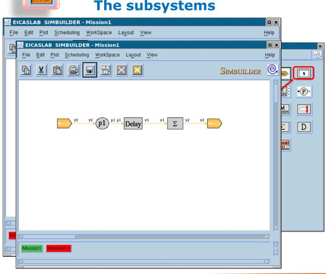
You can simplify the representation of your system by collecting parts of your block diagram in a block called **Subsystem**.
