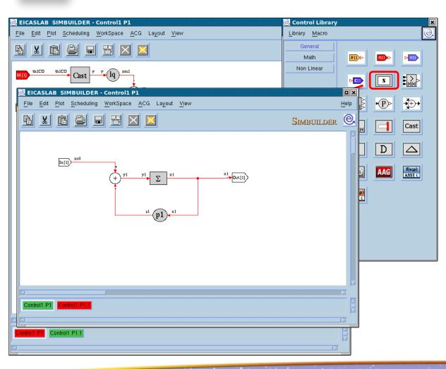
You can simplify the representation of your system by collecting parts of your block diagram in a block called **Subsystem**.
